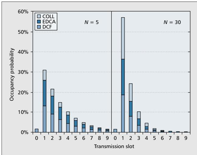
■ Figure 5. Per-slot occupancy probability — AC\_BE vs. DCF.
