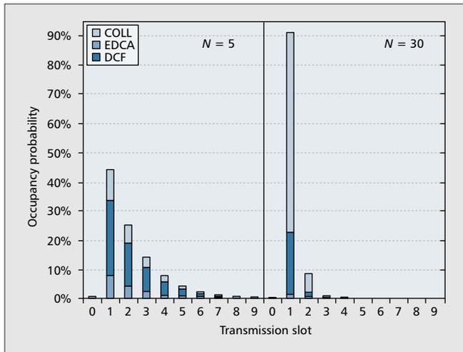
■ Figure 8. Per-slot occupancy probability —  $CW_{min}$  and  $CW_{max}$  differentiation.
