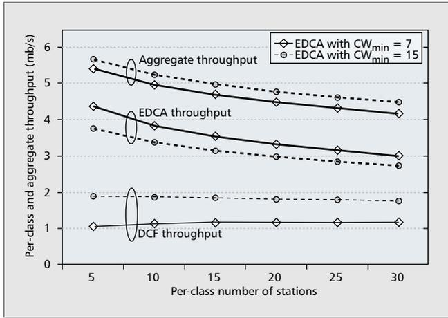
Figure 1. DCF vs. EDCA throughput with  $CW_{min}$  differentiation.
