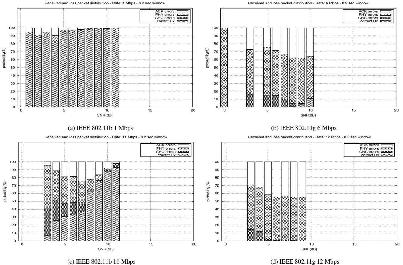
Figure 5. Typical results of the correctly received and loss packet distribution
