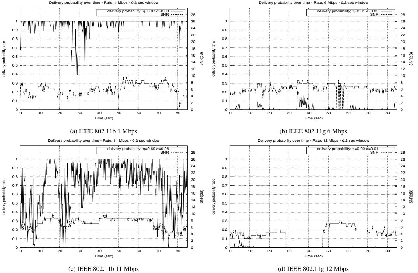
Figure 3. Delivery probability ratio of a typical Mesh Link
