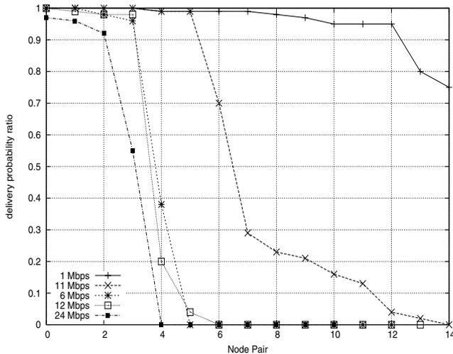
**Figure 4. Delivery probability ratio as function of the node pair**
