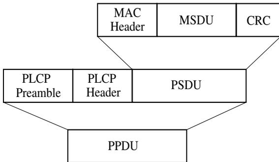
**Figure 1. PPDU IEEE 802.11 frame format**
