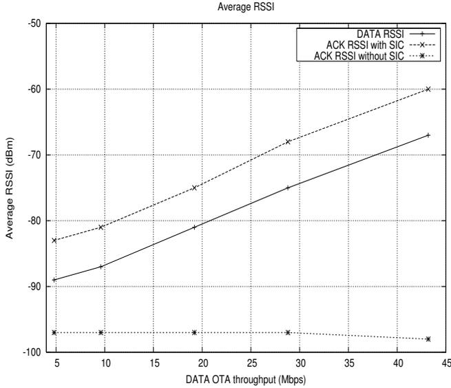
Fig. 4. Average DATA/ACK frame RSSI vs DATA over-the-air throughput
