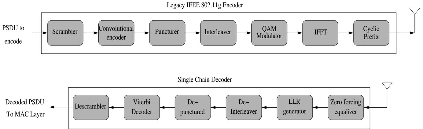
Fig. 3. IEEE 802.11g encoder and single chain decoder of a legacy terminal
