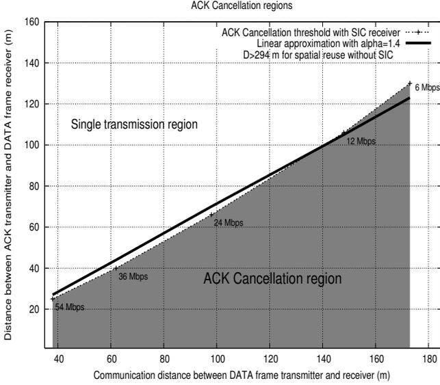
Fig. 5. Link distance for ACK cancellation in IEEE 802.11g mesh networks
