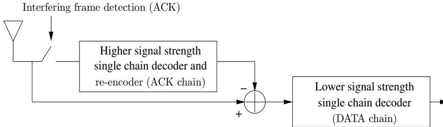
Fig. 2. Interference cancellation: the SIC Receiver in IEEE 802.11
