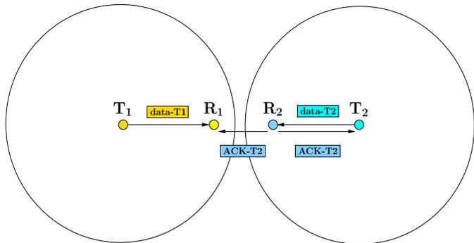
Fig. 1. Hidden ACK Phenomenon: the ACK transmitted from  $R_2$  to  $T_2$  interferes with the transmission from  $T_1$  to  $R_1$
